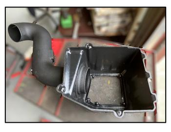
Locate the Volant Intake Duct and insert it into the Volant Intake Box Top and Seal. Orient the parts as shown.
