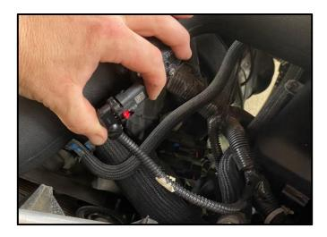
14. Once the MAF Sensor is secured, reconnect the Wire Harness and push the Red Locking tab.
