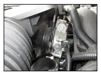
3. Using a 7mm Socket & Ratchet or Wrench, loosen the Hose Clamp connecting the Factory Air Duct to the Throttle Body. This will not be reused.
