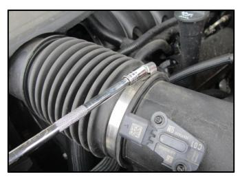
Using a 7mm Socket & Ratchet or Wrench, loosen the Hose Clamp connecting the Factory Air Duct to the Factory Air Box. This will not be reused.
