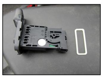
Locate the MAF Sensor removed in from Removal Step 8. Remove the Factory MAF Gasket. This will not be reused.
