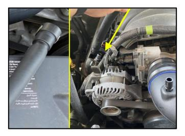
10. Locate the Hose and Quick Connect Fitting. Press the fitting into one end of the hoses, as shown on the left.
