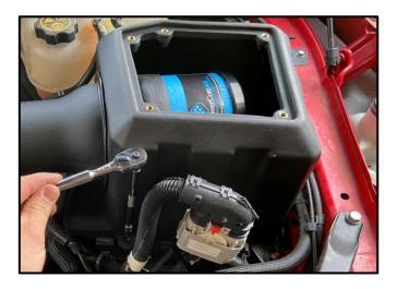
Locate the 3 Screws from Removal Step 7.
