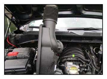
6. Rotate the Factory Air Duct until it is vertical. Then, lift the Factory Air Box up from the bracket located on the vehicle's engine and remove the Factory Air Duct. This will not be reused.
