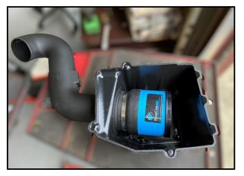
Locate the Volant Air Filter (PowerCore shown).
