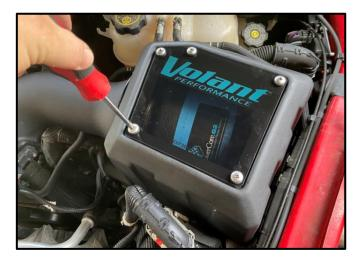
Locate the 5 screws and rubber washers from Install Step 1. Using a Phillips screwdriver, install the Volant Lid.
