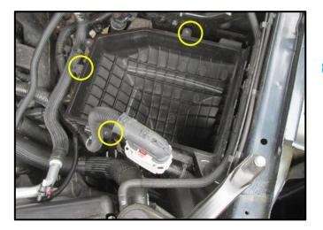
8. Remove the Factory Air Box Top and Filter. These will not be reused.
