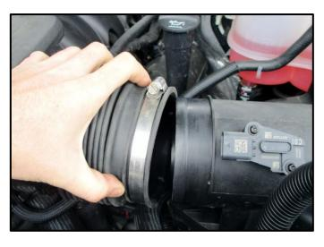
5. Pull the Factory Bellows on the Factory Air Duct off the Factory Air Box.
