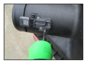
Using a T20 Torx Driver, remove the Factory MAF Screws. Carefully remove the MAF Sensor and store it in a safe location. It will be reused in Installation Step 12. The screws will not be reused.
