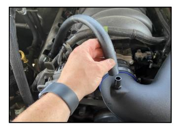
11. Route the hose to the fitting in the Air Intake Duct, as shown.
