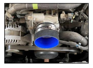
**6.** Locate either the Ø4in to Ø3.5in Reducer (5.3L) (shown) or Ø4in Hose (6.2L). If installing on a 5.3L engine, slide the smaller Hose Clamp from the Hardware Kit on the smaller side first (shown). Place the other clamp over the other side. The hose clamps should be loose at this time.
