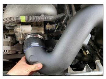
Insert the Volant Air Duct into either the Ø4in to Ø3.5in Reducer (5.3L) (shown) or Ø4in Hose (6.2L), depending on application.
