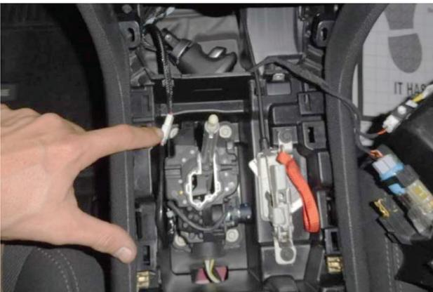
14. Route harness to driver side of shifter housing. Place stock handle into empty space in front of shifter housing under tray (removed step 11). Challenger models have an empty space just forward of shifter housing.
