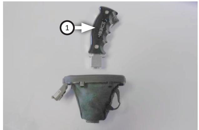
17. With boot inverted, insert **pistol grip (1)** into boot, orienting it as shown.
