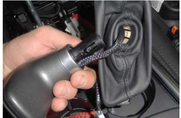
9. Separate shift boot from shift handle and wire harness.
