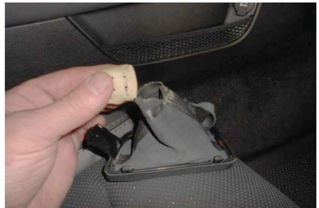
10. The shift boot collar is attached to shift boot with glue. Separate collar from boot, being cautious not to tear boot.
