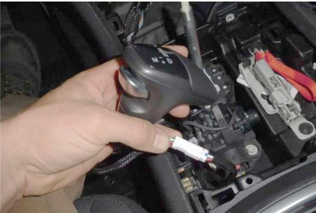
13. The factory shifter features a computer chip for illuminated gear select indicator. If disconnected, the vehicle ECM will not see it and an error light will be generated. To remedy this, plug factory shift handle back into factory connector.
