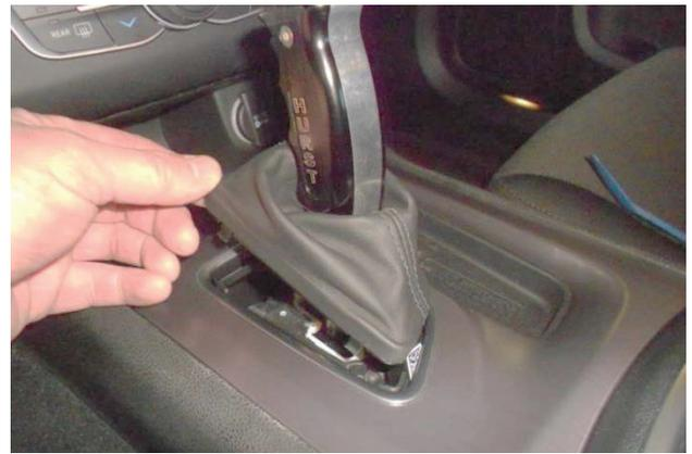
21. Clip shifter boot back into bezel. Shift through all positions to ensure proper installation.
