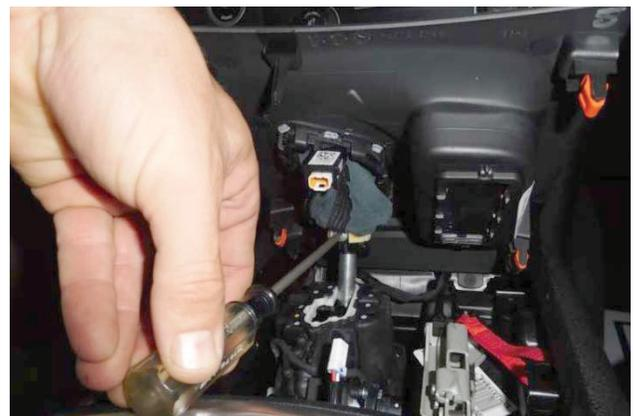
5. Remove factory set screw located at base of shift handle. Pull straight up on shift handle to remove handle and bezel assembly.
