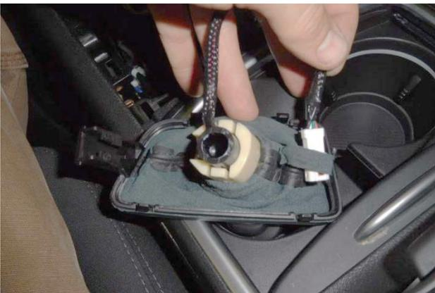
7. Detach shift handle wire harness from mount on shift boot then pull it through boot loop.
