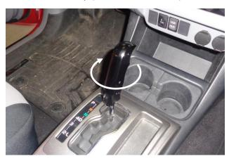
3. Thread the handle body all the way on to the shifter stick.
