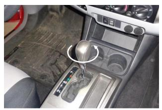
Turn off your vehicle's ignition and set the parking brake. Remove the stock shifter handle by rotating it counter-clockwise on the shifter stick.
