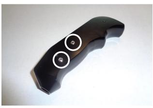
2. Thread the 4 set screws (Item 5) into the shifter handle body (1) until they are almost flush with the handle body. (Two screws each side.)
