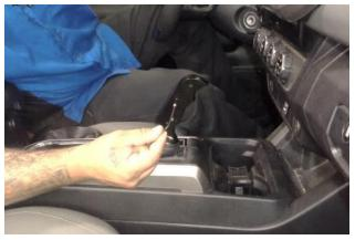
7. Install the six set screws (5) in the shifter handle—three screws on each side. Align the handle as desired, then tighten the set screws.
