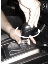
Separate the trim ring from the shifter handle by pushing down on both sides of the shifter boot. Then rotate the shifter handle counter-clockwise to remove it from the stick.
