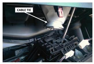
4. Push the shifter boot to underneath the console. Cut the cable tie securing the trim ring in the shifter boot and remove the ring.
