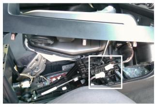
On the passenger side of the console, find and disconnect the electrical connector. Then lift the shifter boot off the shifter stick. NOTE: Leave the emergency brake connected to its boot.
