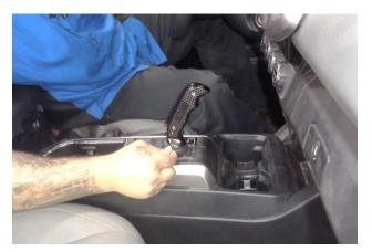
8. Install the two shifter handle covers (2) and (3) using the four flat head screws (4) – two screws on each side.
