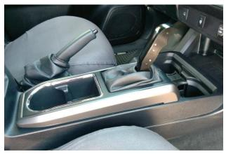
6. Carefully lower the shifter handle over the shifter stick. Reconnect the electrical connector, then snap the center console back into its base.
