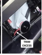
5. Work the shifter handle (item 1) up through the boot until the its opening surrounds the notch at the base of the handle. Use the supplied cable tie to secure the boot to the handle. Trim the cable tie.
