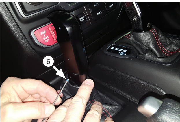
25. Remove SHS screws (x2) (3) and left shifter plate (2) from transfer case handle. Apply medium-strength thread locking fluid to extended tip screw (6) then install into transfer case handle as shown.
