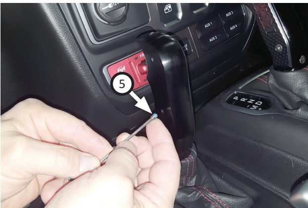
26. Apply medium-strength thread locking fluid to set screw (5) then install into transfer case handle as shown.
