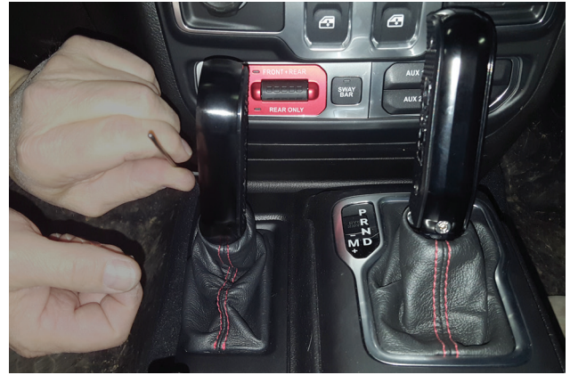
27. Reinstall screws and left shifter plate (removed step 25) onto shift handle body.
