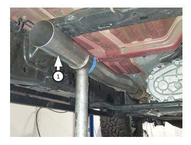
7. Place hanger mount (removed step 1) and **clamp (3)** onto **muffler (2)** then connect it to inlet pipe, inserting wires into hangers. Securing assembly by bolting mount to vehicle frame and tighten clamp.
