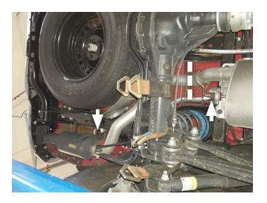
4. Loosen ball clamp from resonator inlet. Remove remaining hanger mount from vehicle frame then with help, remove resonator section from vehicle. Retain clamp and mount for later use.
