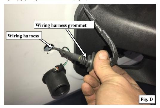
WARNING: REMOVE WIRING HARNESS COMPLETELY FROM THE OE TAILGATE, THROUGH THE EXTERIOR HOLE. FAILURE TO DO SO MAY RESULT IN DAMAGE TO THE WIRING HARNESS.
